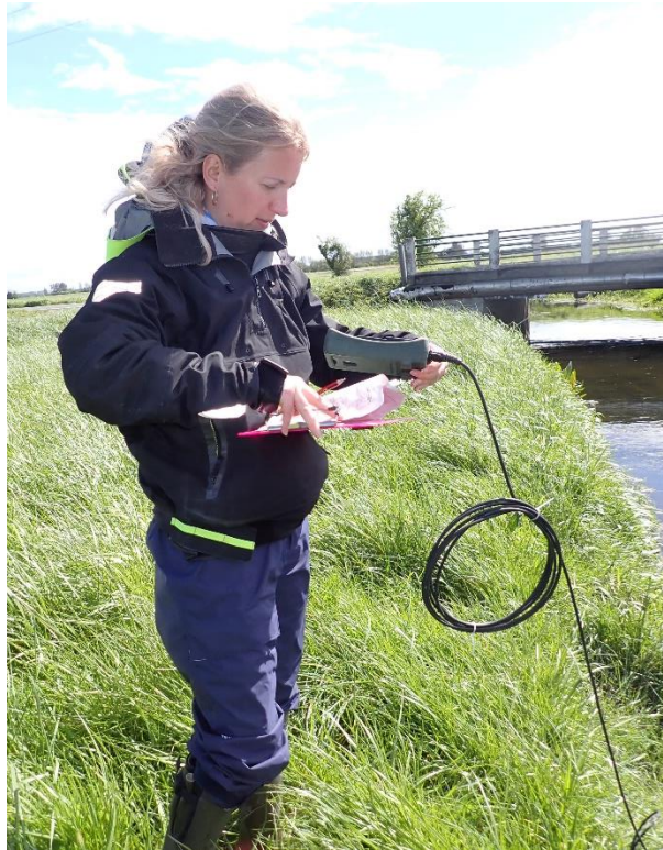
Figure 74 : Environmental parameters being recorded using the probe on the Canal de Retz
